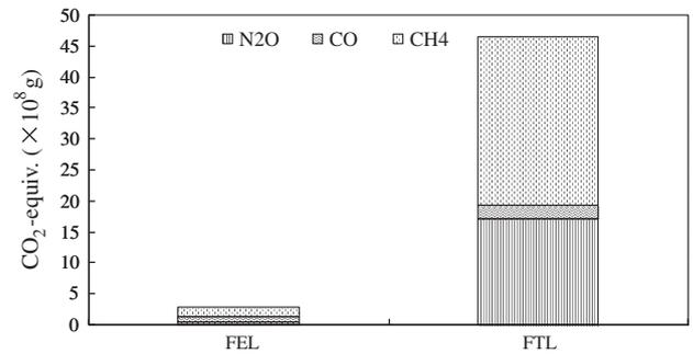
Fig. 9. Life cycle CO<sub>2</sub>-equiv. emissions of the solar BHP system in FEL and FTL operation strategy.
