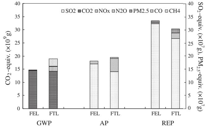
Fig. 8. The life cycle CO<sub>2</sub>-equiv., SO<sub>2</sub>-equiv. and PM<sub>2.5</sub>-equiv. emissions and GWP, AP and REP structures of the solar BHP system in FEL and FTL operation strategies.
