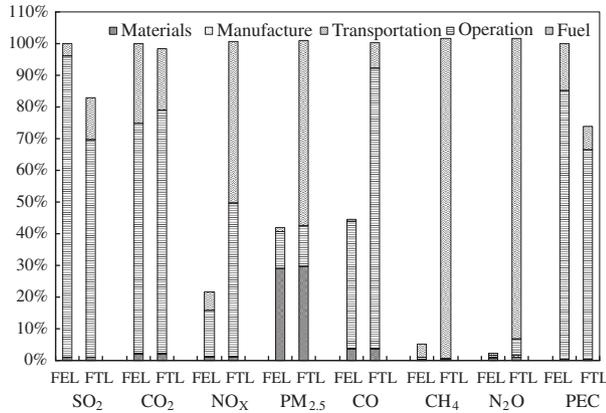
Fig. 7. The normalized life cycle pollutant emissions and PEC results and the LCI structures for the solar BHP system in FEL and FTL operation strategies.
