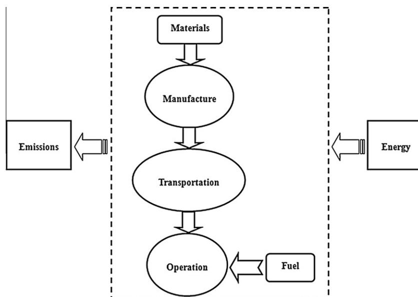
Fig. 2. System boundary of the LCA analysis for the solar BHP system.
