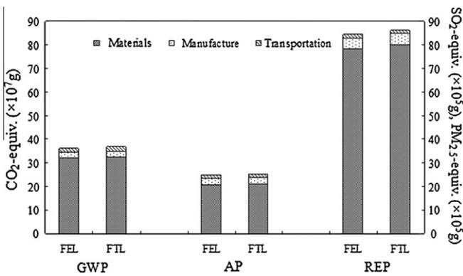
Fig. 11. The life cycle CO<sub>2</sub>-equiv., SO<sub>2</sub>-equiv. and PM<sub>2.5</sub>-equiv. emissions in the materials, manufacture and transportation stages of the solar BCHP system in FEL and FTL operation strategies.
