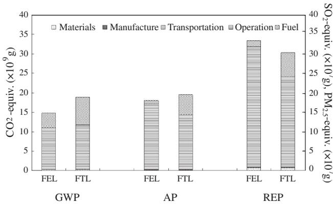
Fig. 10. The life cycle CO<sub>2</sub>-equiv., SO<sub>2</sub>-equiv. and PM<sub>2.5</sub>-equiv. emissions and LCI structures of the solar BCHP system in FEL and FTL operation strategies.
