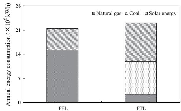
**Fig. 6.** The annual operation energy consumption of the solar BHP system in FEL and FTL operation strategies.
